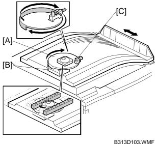
Half turn detection is performed through a combination of two components: the slip disc [A] and half turn sensor [C].
